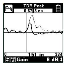
If the circuit being tested is stable (no intermittent faults), then the minimum, maximum and "live" traces should appear as a single trace.
